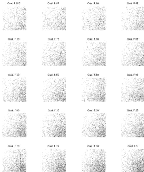
The magnitude of frequency domain coefficients of an interpolated, JPEG compressed body CT image at several quality factors. The darker the area the lower the magnitude. As expected, with the increase in compression, there are more (higher frequency) coefficients of lower magnitude.
