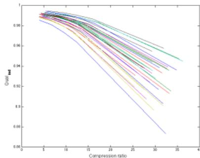
Rate distortion curves for 60 JPEG Body CT images corresponding  $Qual_{ind}$
