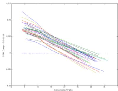
SSIM quality score differences between interpolated compressed and compressed 60 Body CT images as several compression ratios. **The difference becomes negative! It means that the compressed interpolated images seem to be of better quality their compressed (not-interpolated) counterparts!!!**
