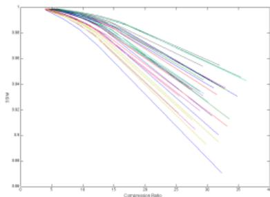
Rate distortion curves for 60 JPEG Body CT images corresponding SSIM.
