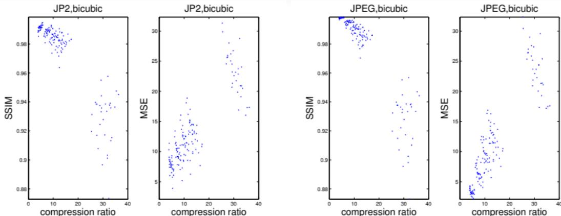
Rate distortion plots corresponding to Body CT images. With higher compression ratio the quality of images (compressed-interpolated) gets worse according to the most common measures of image fidelity.
