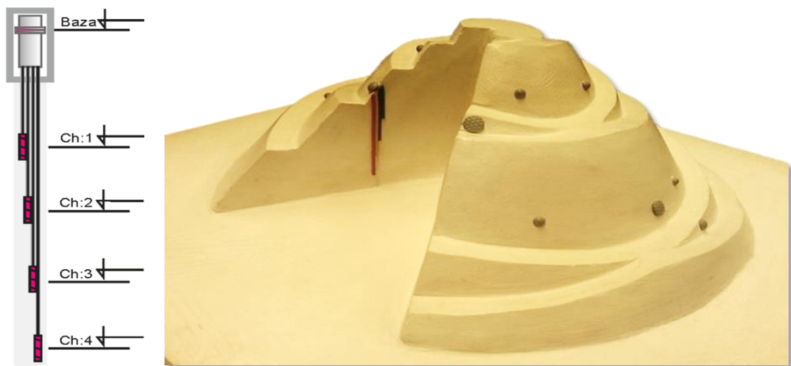
Fig. 5. Details of vertical displacement measurements.
