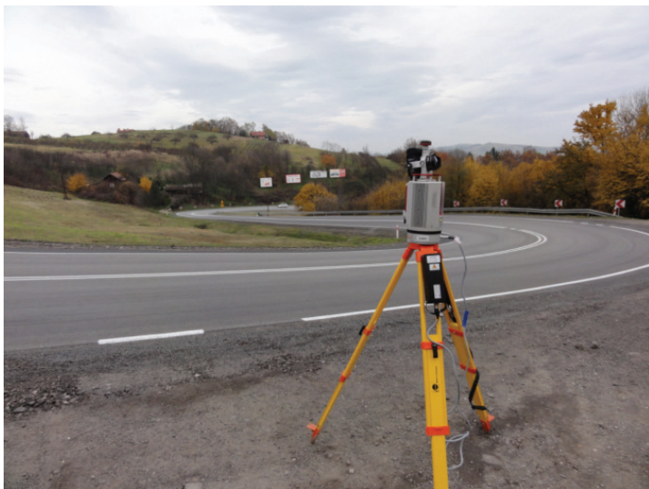
Fig. 4. Measurements with a laser scanner on the Just – Tęgorzorz landslide [16]
