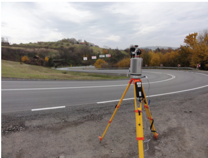
Fig. 4. Measurements with a laser scanner on the Just – Tęgorborze landslide [16]
