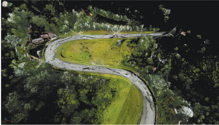
Fig. 6. Three-dimensional terrain model DK 75 on the Just-Tęgorbże landslide [16]
