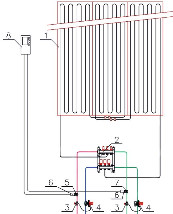
Fig. 4.34. Example of heating and cooling combined into one system [29]; 1 – wall panel, 2 – manifold, 3 – balancing valve, 4 – differential pressure regulator, 5 and 7 – thermostatic valves, 6 – thermal actuator, 8 – controller
