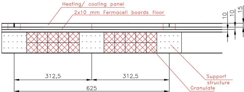
Fig. 4.32. Dry system in-floor heating [29]
