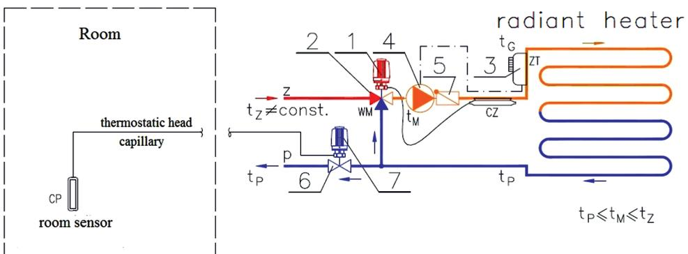
Fig. 4.15. Room air temperature control system with thermostatic head and capillary [26]:
