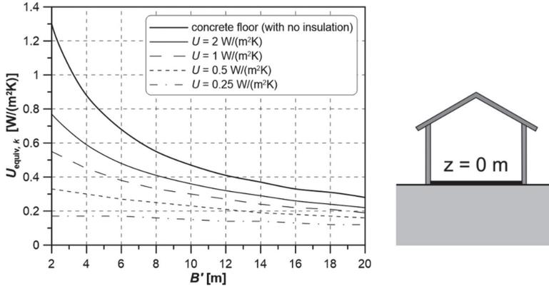
Fig. 2.4. Equivalent heat transfer coefficient of floor at ground level — based on [1]
