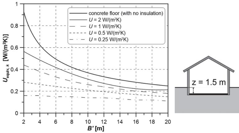
Fig. 2.5. Equivalent heat transfer coefficient of the heated underground floor with the floor slab located 1.5 m below the ground level — based on [1]
