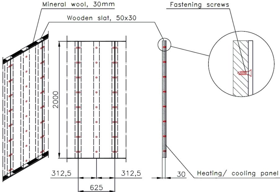
Fig. 4.30. Heating panel mount to wall [29]
