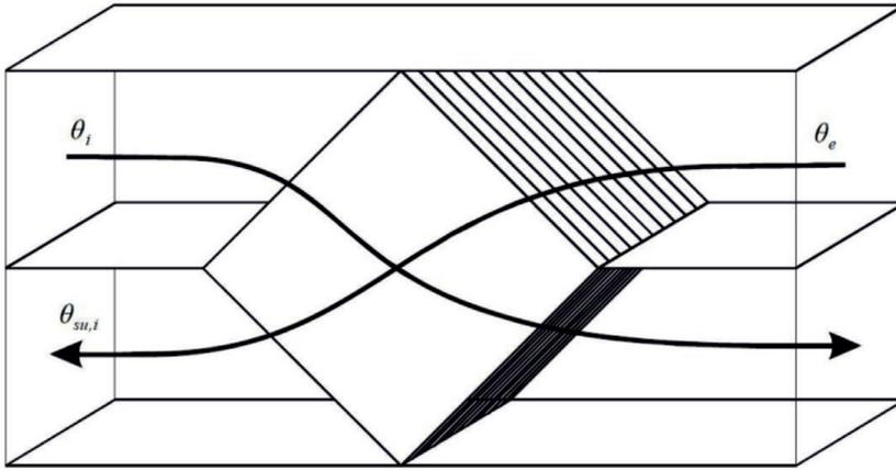
Fig. 2.9. Heat recovery by a plate heat exchanger [3]
