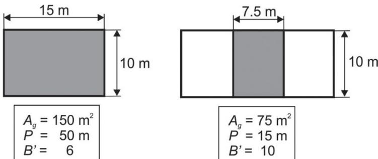
Fig. 2.8. Determination of characteristic dimension  $B'$  [1]
