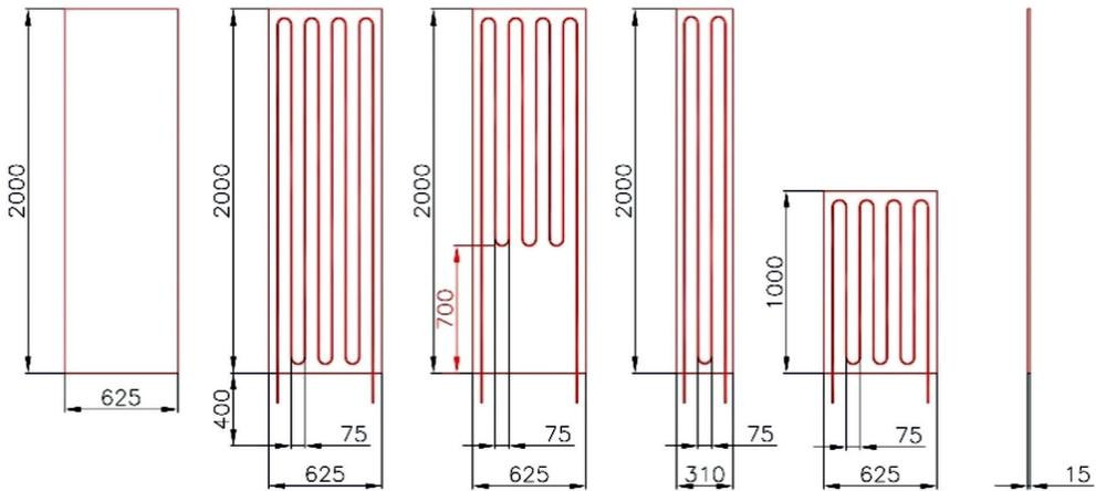
Fig. 4.29. Dry system heating panels [29]
