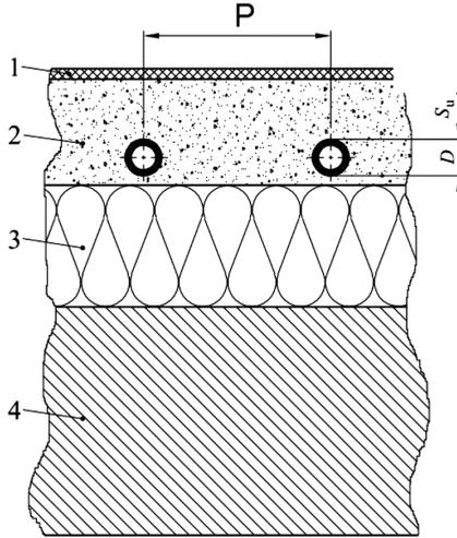
Fig. 4.4. System with under-screed ducting (type B) [16];
