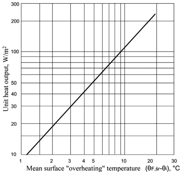
Fig. 4.5. Surface heat transfer characteristics [16]
