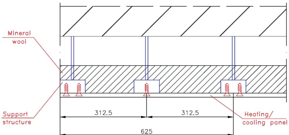
Fig. 4.33. Dry system ceiling heating [29]
