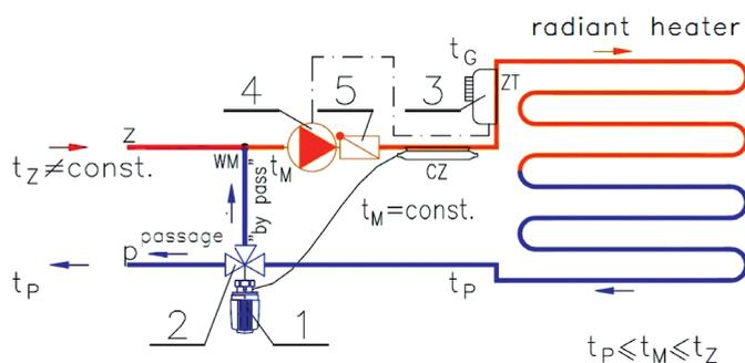
Fig. 4.11. Thermostatic temperature control system with a three-way valve at return [23]:
