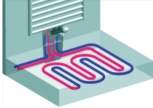
Fig. 4.44. Connection unit with floor heater [29]
