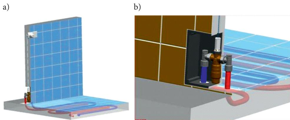
Fig. 4.40. In-floor heating control system with double temperature adjustment [29];
