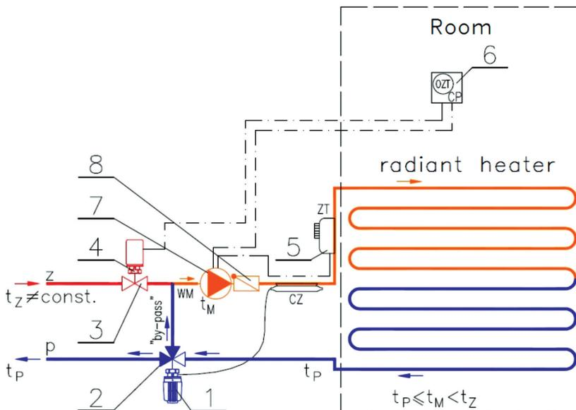
Fig. 4.18. Room air temperature control system with electrical controller [27]:
