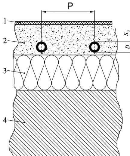
Fig. 4.3. System with in-screed ducting (types A and C) [16];
