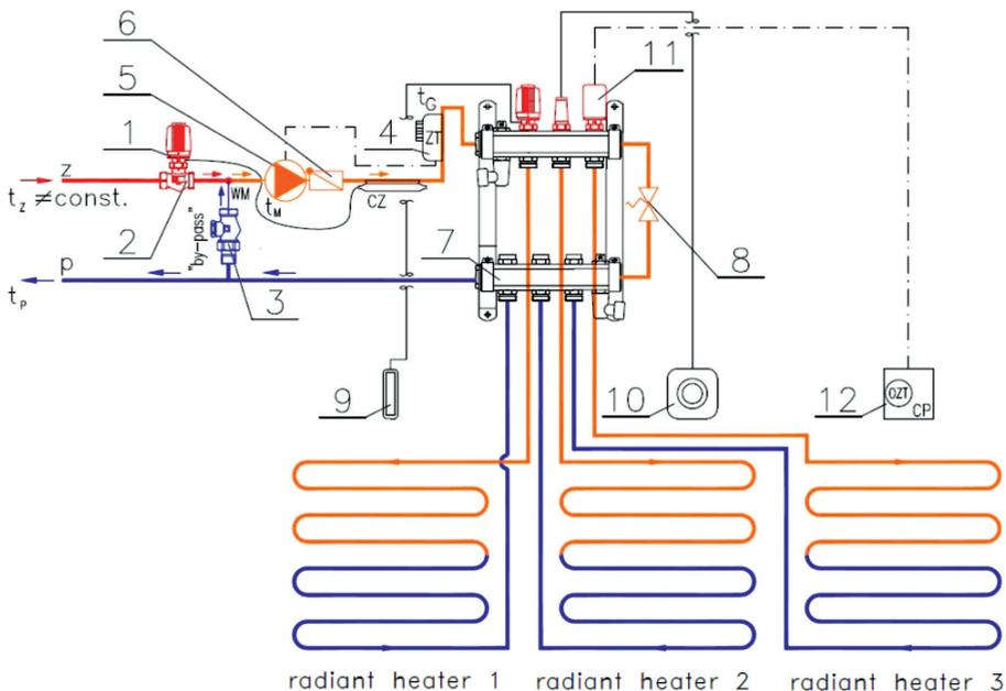
Fig. 4.23. Temperature control system of radiant heating with multiple heating circuits [30]: 1 – thermostatic head with contact sensor, 2 – straight-way thermostatic valve, 3 – bypass control valve, 4 – safety switch, 5 – circulation pump, 6 – check valve, 7 – floor heating manifold, 8 – relief valve, 9 – thermostatic head with remote sensor, 10 – thermostatic head with remote setter, 11 – thermal actuator, 12 – electronic (or electric) controller
