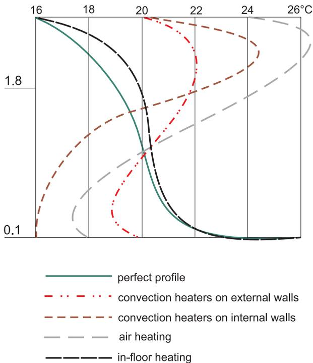
Fig. 4.1. Temperature profile for various heating types [12]
