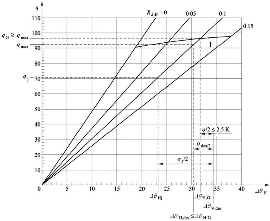
Fig. 4.8. Determination of design temperature difference  $\Delta\theta_{H,des}$  and temperature drop  $\sigma_j$  for the  $j$ -th rooms with different loads [17]
