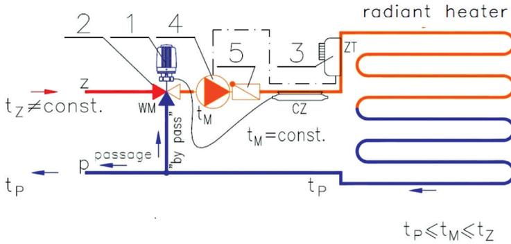
Fig. 4.13. Thermostatic temperature control system with a three-way valve at feed [24]:
