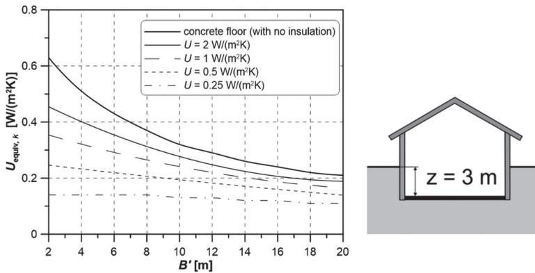
Fig. 2.6. Equivalent heat transfer coefficient of the heated underground floor with the floor slab located 3.0 m below the ground level — based on [1]
