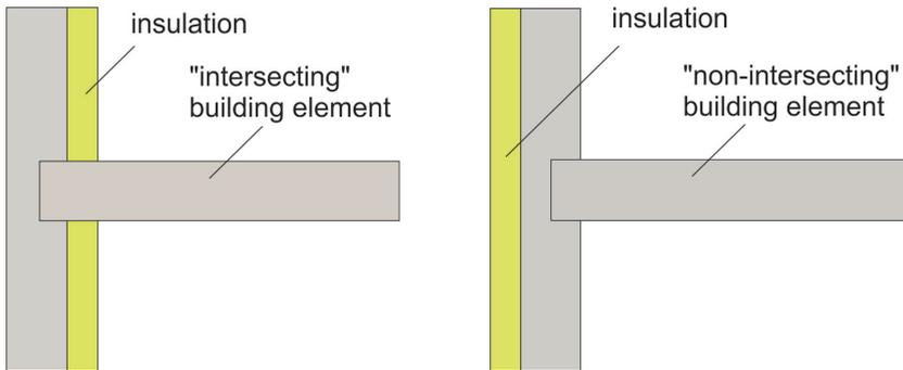
Fig. 2.3. Insulation “intersecting” and “non-intersecting” building elements [1]
