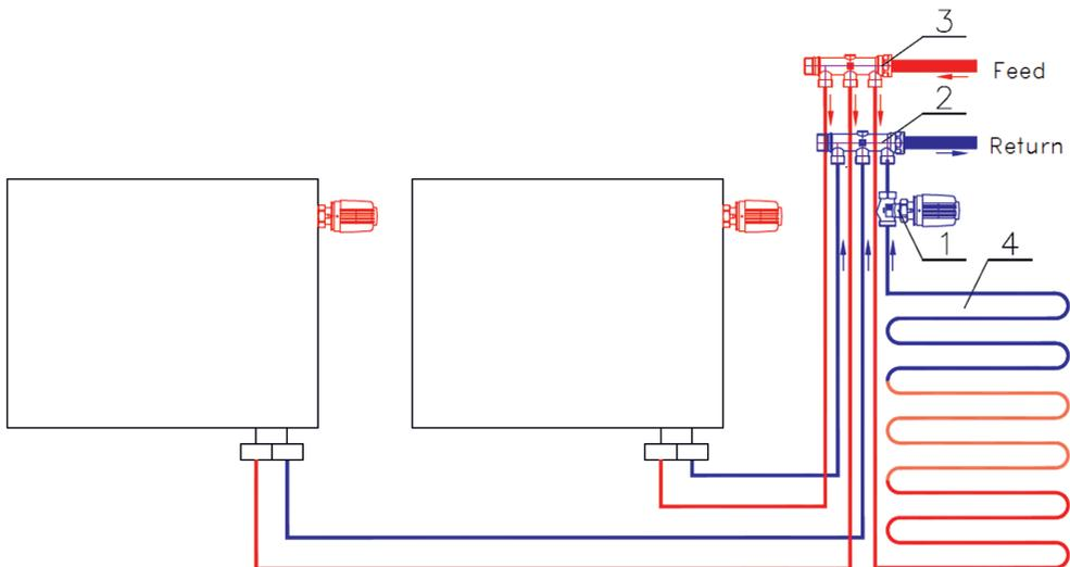
Fig. 4.38. Floor comfort system with panel radiators with incorrect RTL connection [34];
