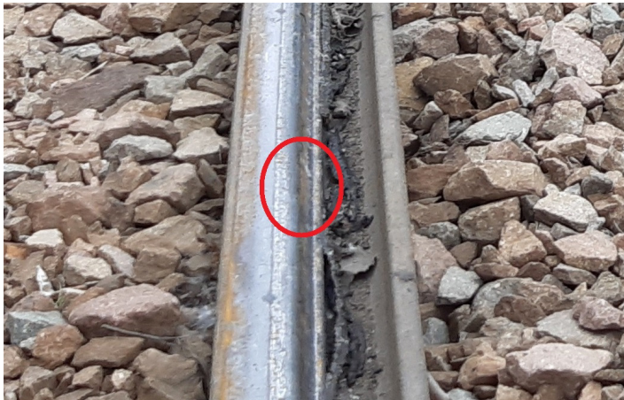
Fig. 4. Lateral wear of the outer rail head on a curve with a radius of 30 m (red - worn part of the rail) [own study]
