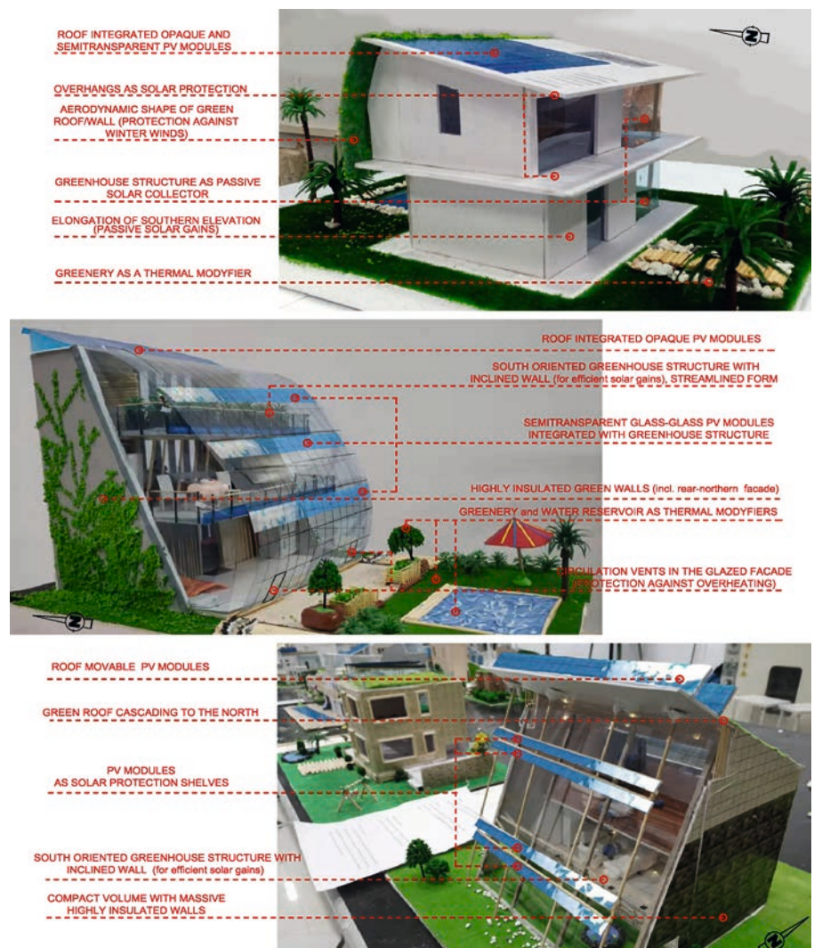
Fig. 5. Selected final designs of one-family solar building with solutions corresponding to the project goals (photos by the author)
