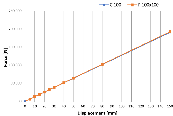
Fig. 9. Results of force difference for different reinforcements upon displacement (own elaboration)
