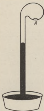
FIG. 28.—Proof that oxygen yields its own volume of sulphur dioxide.
