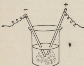
FIG. 108.—Making a colloidal solution of gold.
