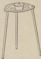
Fig. 120.—Covered Crucible Supported on a Tripod.
