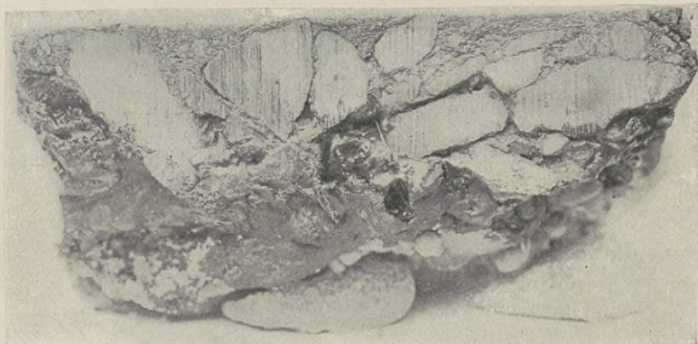
FIG. 100. Section Showing Uneven Penetration.
