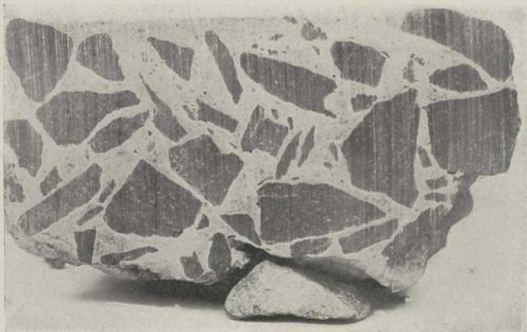
FIG. 136. Section of Cement-Concrete Pavement Constructed by the Grouting Method.
