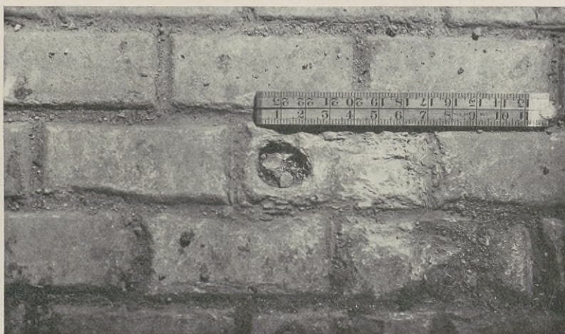
FIG. 163. Blow-hole in Slag Block.
