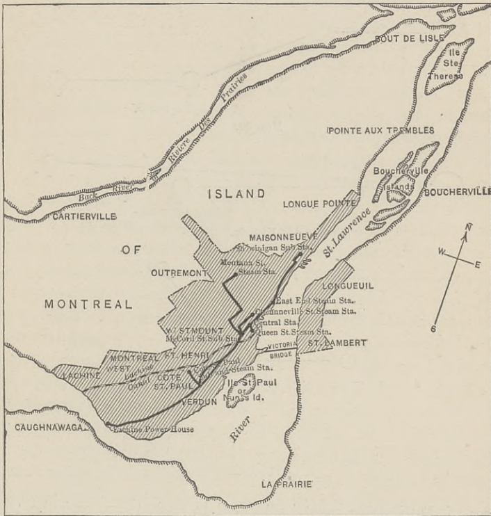
FIG. 65.—Area of Electrical Distribution at Montreal.
