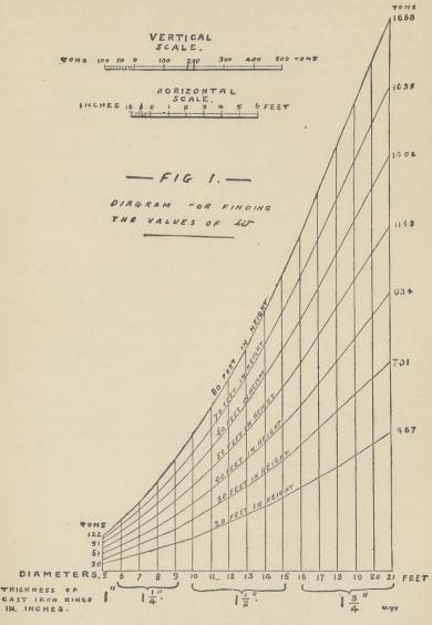
Note.—The weights in the diagram are calculated on the assumption that the hearting of the cylinder is Portland cement concrete. If brickwork, the weights will be about 16 per cent. less for picked stock bricks set in Portland cement mortar.
