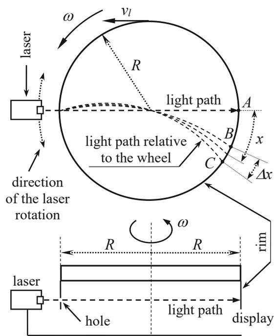
**Fig. 1.** Measuring system of the one-way light speed
