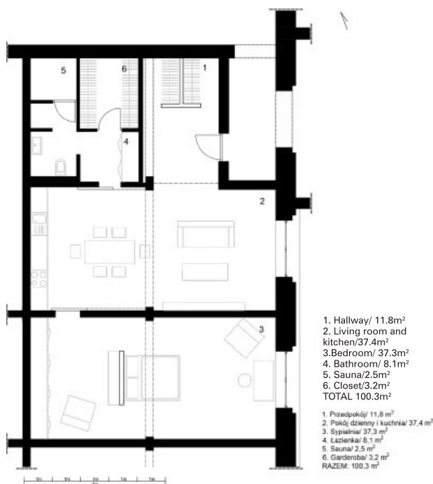
III. 17. Plan of floors 1-3 of the Spichlerz building following adaptation (type 2) (author’s drawing based on available Medusa Group documentation)
