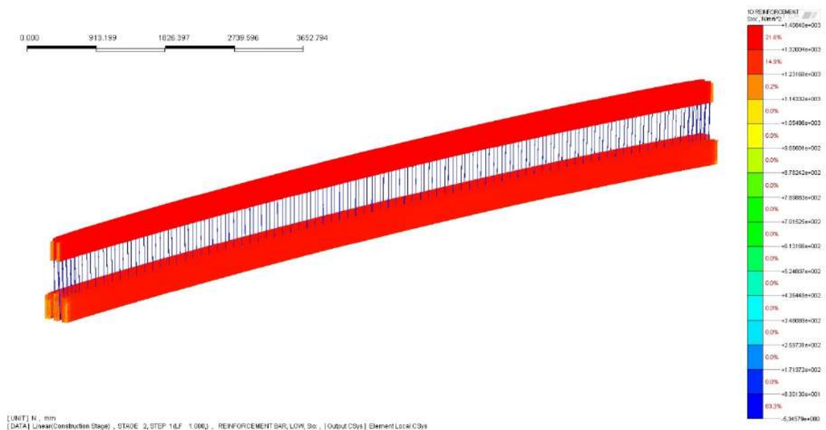
Fig. 8.6: Stress in pre-stressing strands
