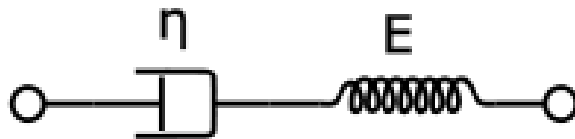
Fig. 6.3: Maxwell spring – dashpot model
