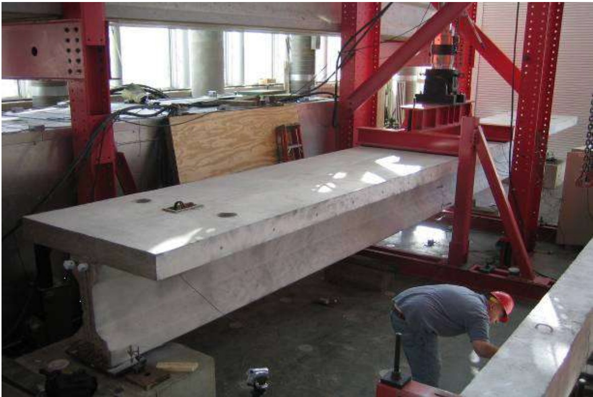
Fig. 2.3: HSC composite girder [Choi, 2006]
