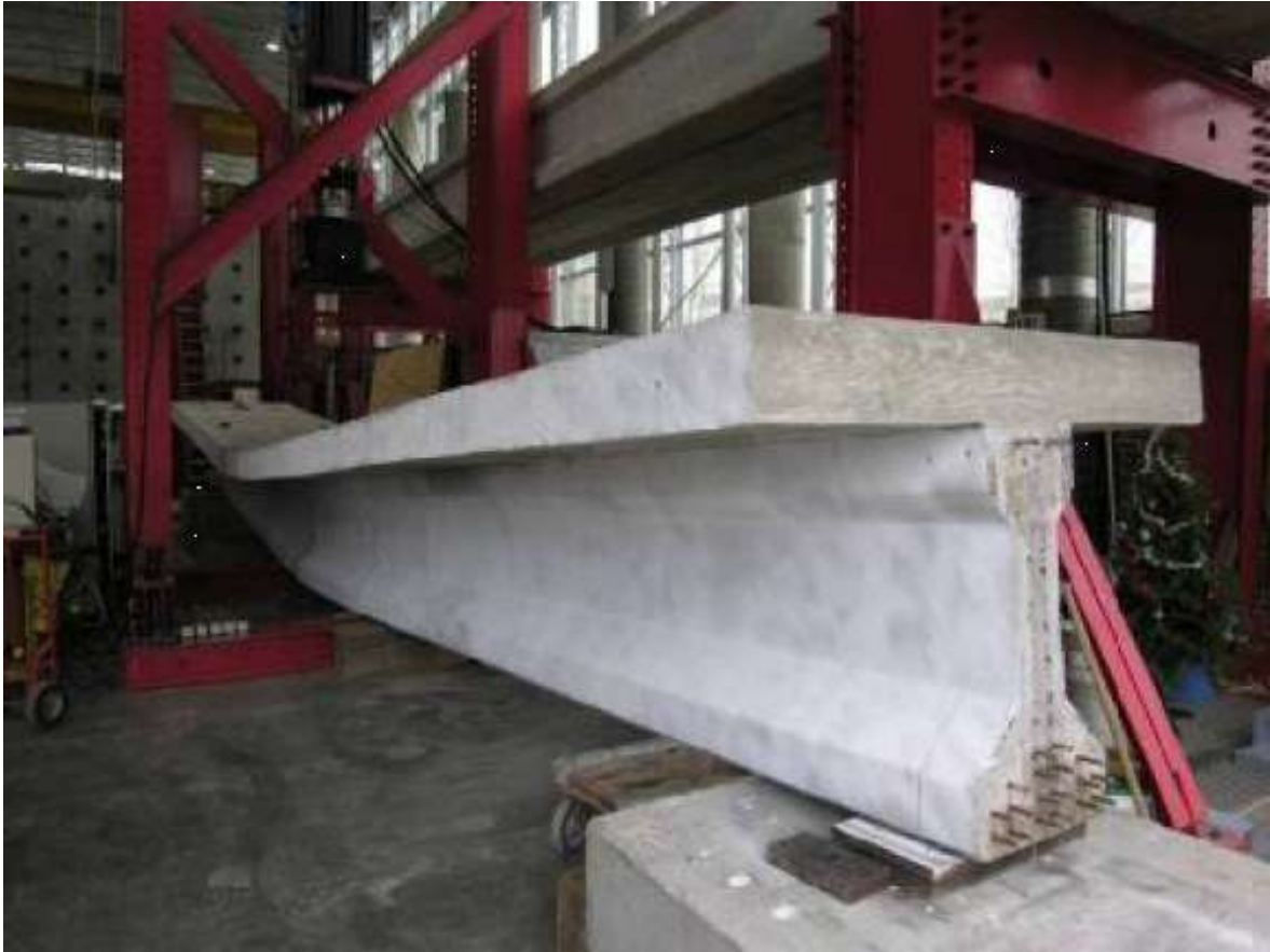
Fig. 2.1: Composite concrete-concrete girder [Halicka, 2007]
