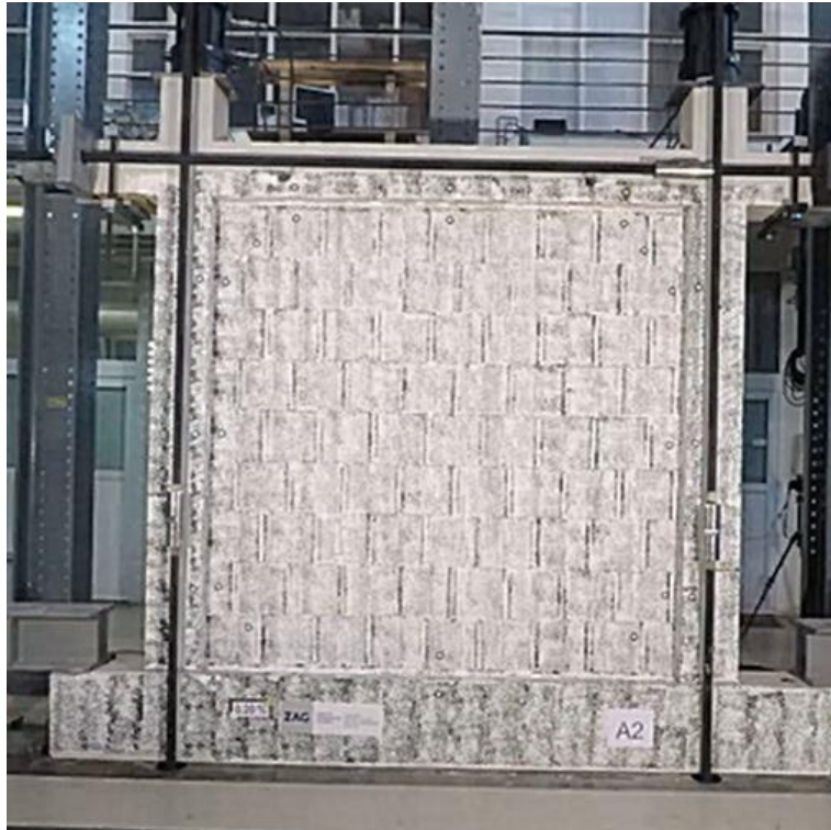
Figure 4.23. View of Frame A at the end of horizontal loading test – 1.6% drift ratio.
