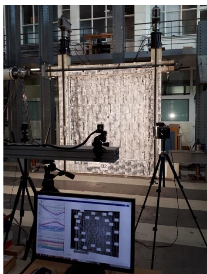
Figure 4.21. Utilization of the DIC method on Frame B.
