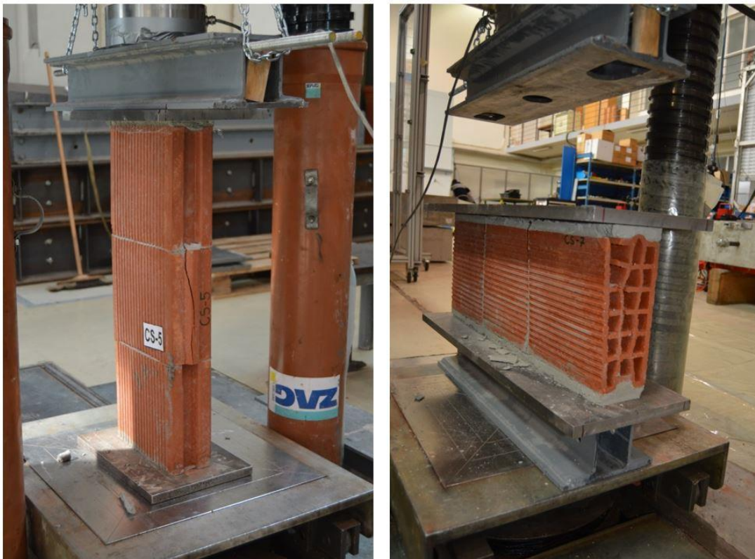
Figure 4.5. Failures on the compressive specimens; vertical (left) and horizontal (right).
