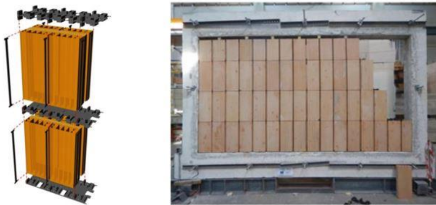
Figure 3.31. Special design blocks details (left) and construction process (right) [adapted from Vailati et al. (2016, 2018)].
