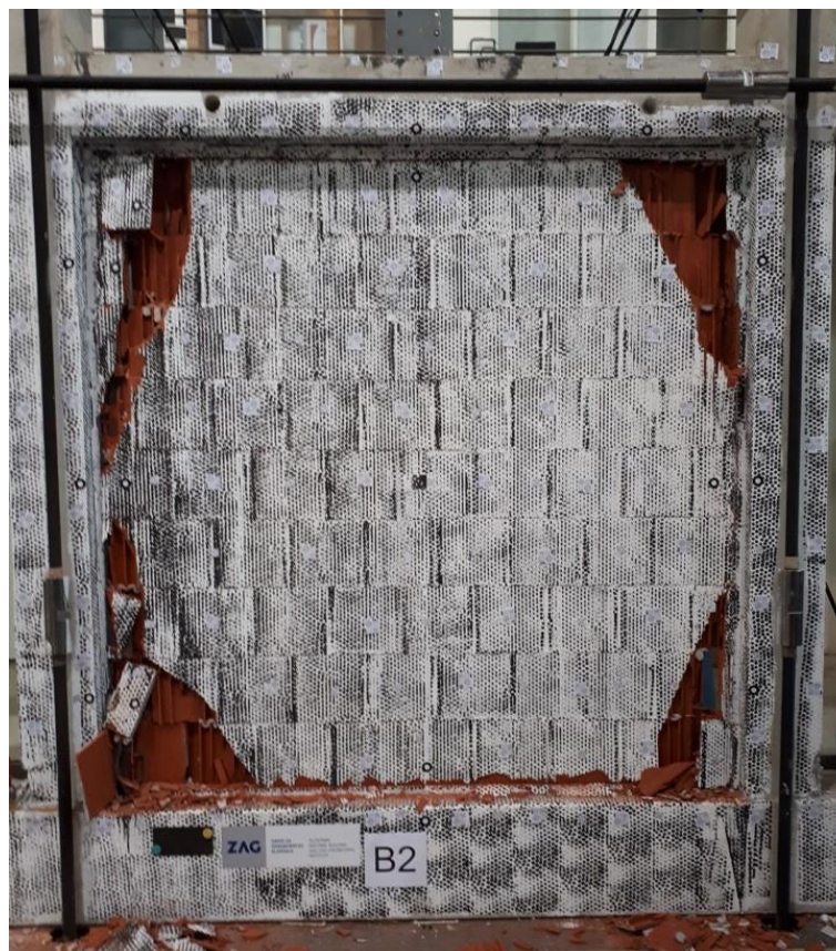
Figure 4.25. View of Frame B at the end of horizontal loading test – 3.5% drift ratio.
