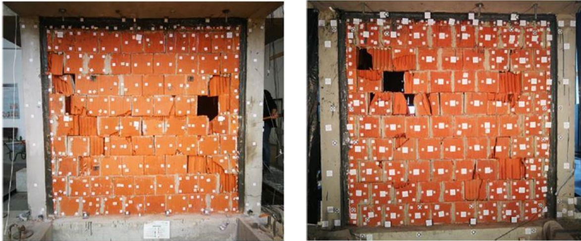
Figure 4.47. Masonry Type B damages at the end of Phase 1; North side wall (left) and South side wall (right).
