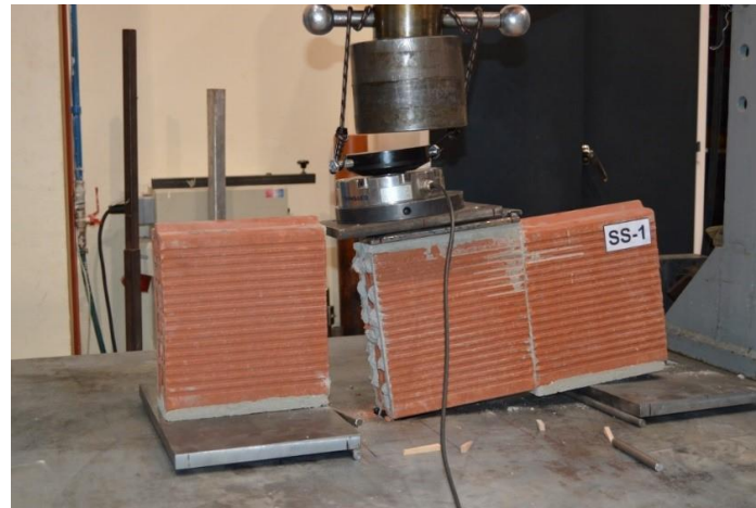
Figure 4.6. Failure on the shear specimen.
