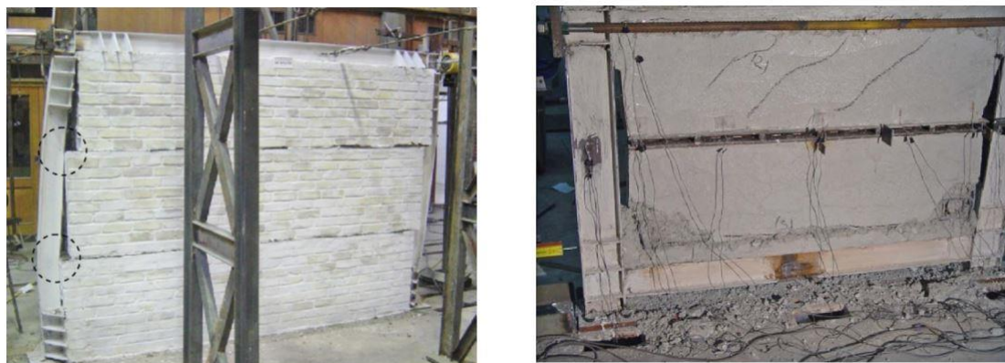
Figure 3.30. Sliding mechanism proposal; initial (left) and upgraded version (right) at the end of tests [adapted from Mohammadi et al. (2011)].
