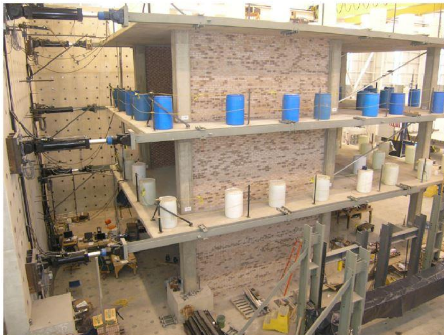
Figure 3.5. Three-story structure before the tests [from Pujol and Fick (2010)].
