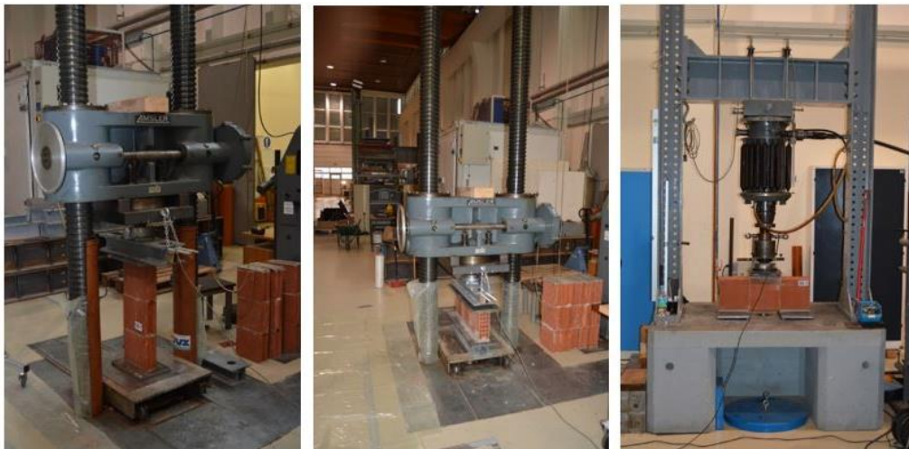
Figure 4.3. Test setups for the triplet specimens; vertical compressive (left), horizontal compressive (middle) and shear (right).
