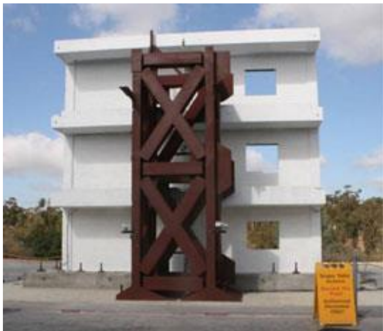
Figure 3.6. Test specimen on the shake table [from Stavridis et al. (2011)].
