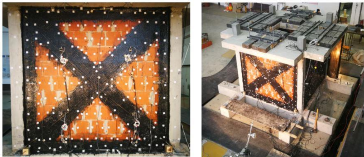
Figure 4.52. FRPU intervention on Type C infills; front (left) and perspective (right) views.
