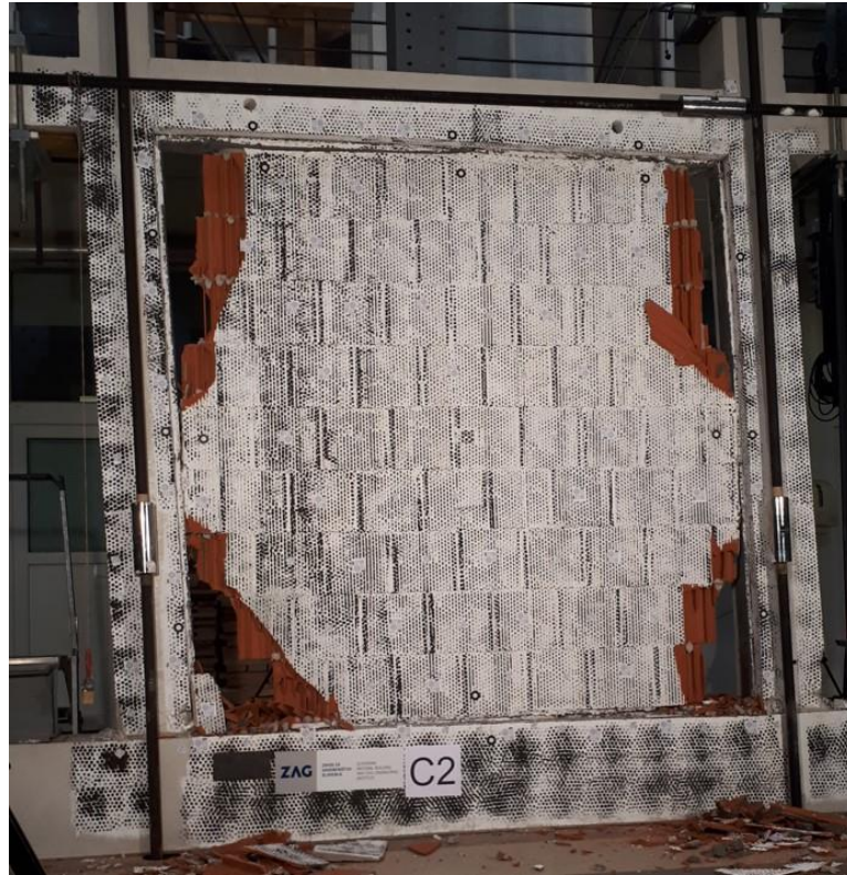
Figure 4.27. View of Frame C at the end of horizontal loading test – 4.4% drift ratio.
