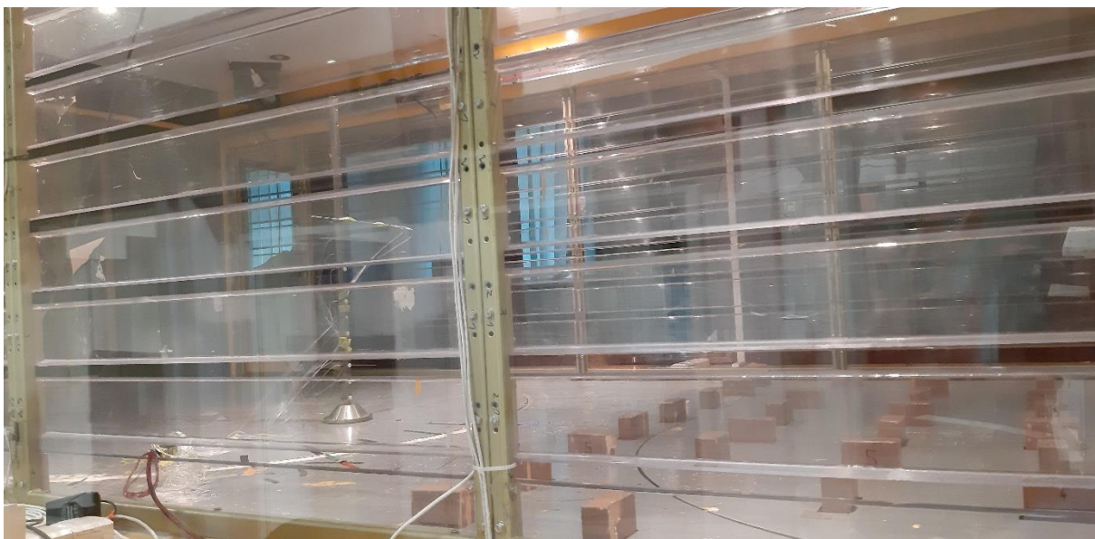
Fig. 3.14. Slotted sidewalls at the wind tunnel of the Wind Engineering Laboratory of Cracow University of Technology
