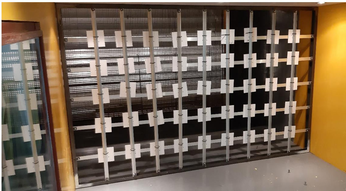
Fig. 3.15. Turbulising net at the Wind Engineering Laboratory of Cracow University of Technology
