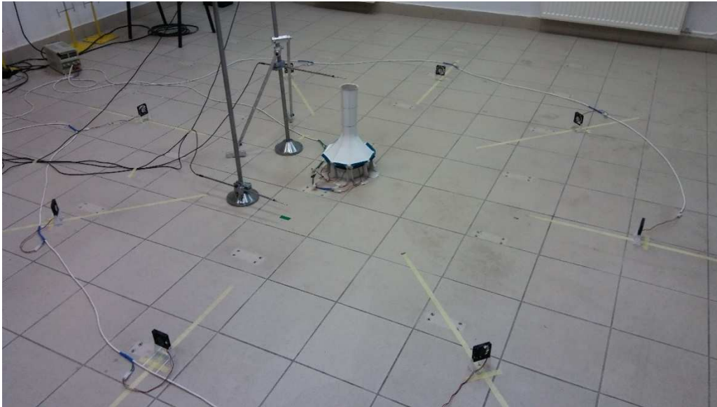
Fig. 8.20: Chimney model (shape A) with inlet fans visible at the base, fan outer ring at a distance of 120 cm from the chimney, and stands with measuring probes 1 and 2
