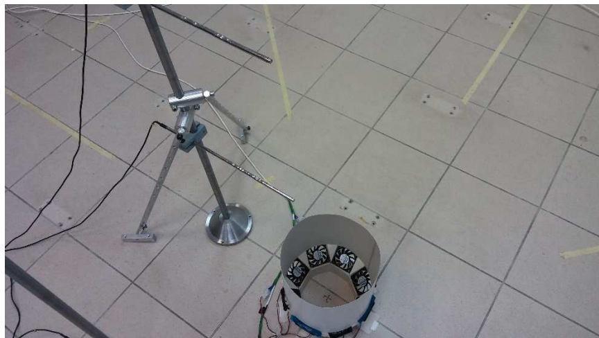
Fig. 8.22: Model of the chimney (shape C) with the position of the inlet fans visible from the inside
