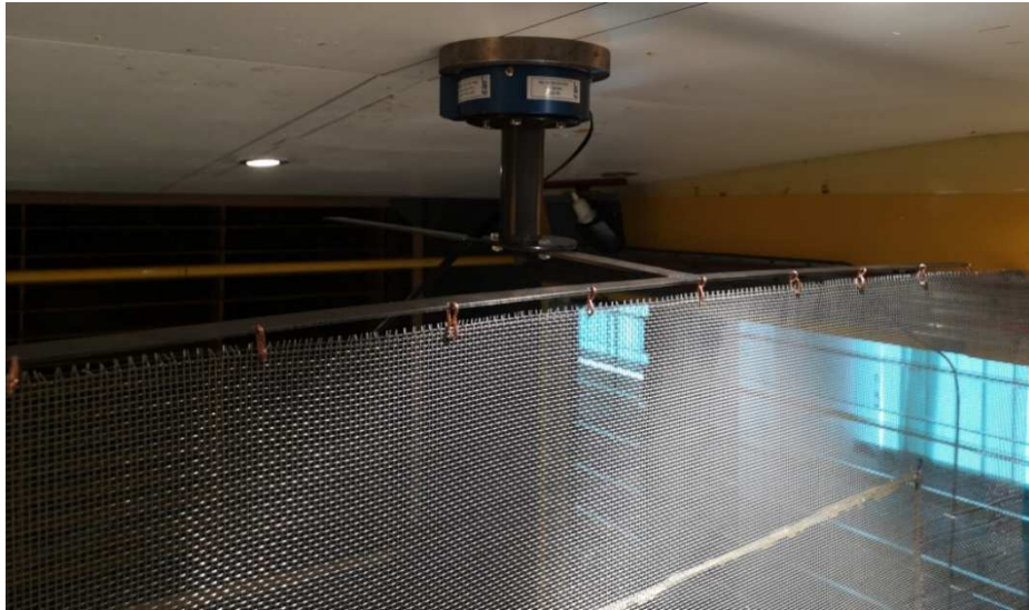
Fig. 9.13 Attachment of the mesh to the aerodynamic balance.
