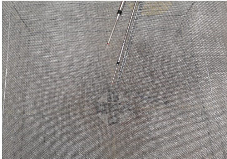
Fig. 9.10 Top view of the ventilation chimney and measuring probes between the mesh.
