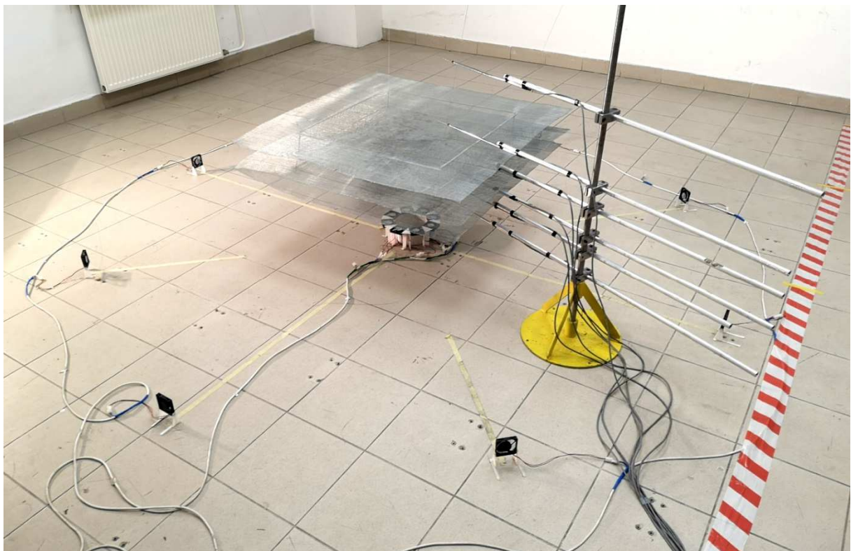
Fig. 9.9. A ventilation chimney with an inversion layer and an outer ring of fans and 6 measuring probes.
