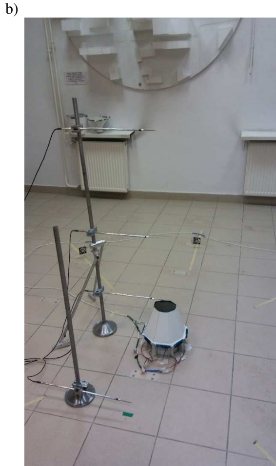
Fig. 8.21: View of the arrangement of hot-wire anemometric sensors on the system model: a) shape A, variant 1 b) shape B, variant 3
