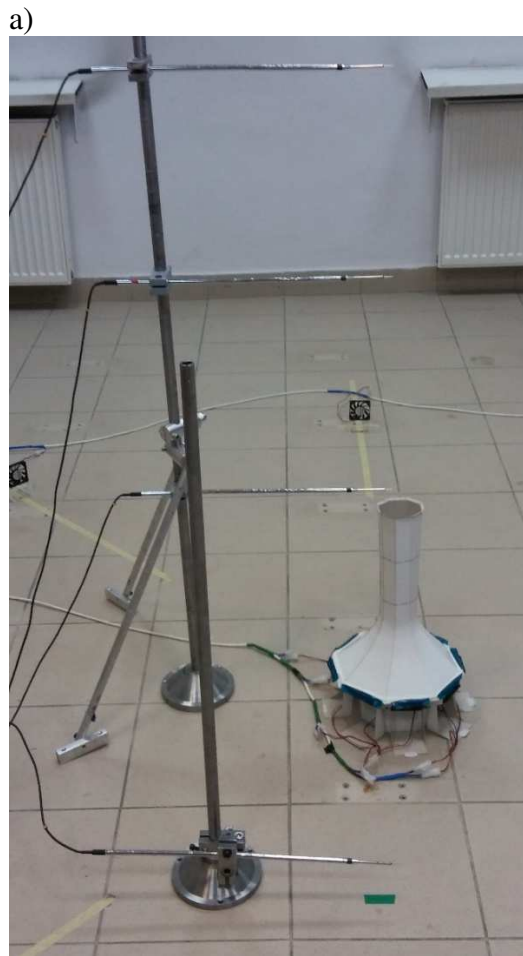
Fig. 8.21: View of the arrangement of hot-wire anemometric sensors on the system model: a) shape A, variant 1 b) shape B, variant 3
