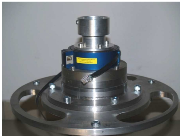
Fig. 9.12. Six-component aerodynamic scale in the test setup (Fot. Ł. Flaga).
