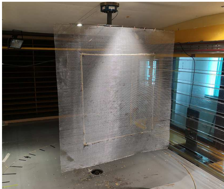
Fig. 9.11 The mesh in the test set up in the wind tunnel.
