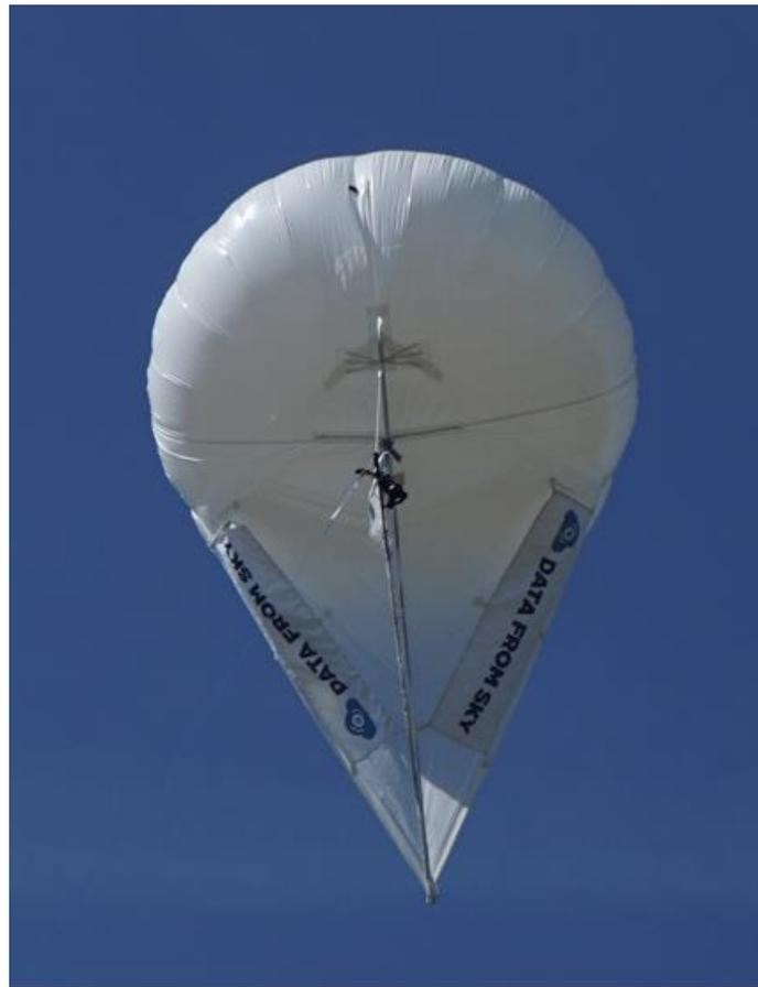
Figure 19: Balloon used for the video detection of the vehicles. Source: [237]
