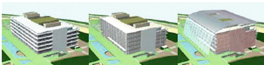
Fig. 8. The influence of shadowvoltaic system on the buildings form: three variants of Itoman City Hall, from the left – basic volume, volume with traditional lamellas, volume with sloped shadowvoltaic system-implemented variant (source: Tochigi & Tsukamoto, 2005)
