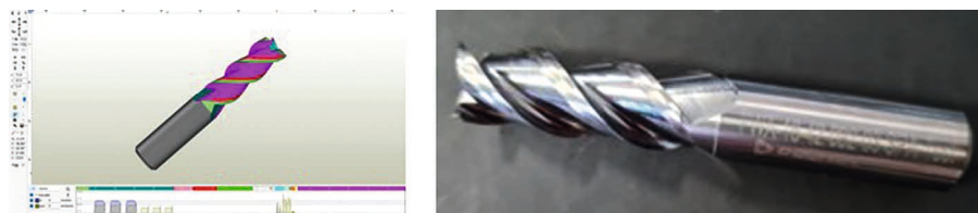
Fig. 7. (a) The design of the tool in NumRoto and its visualisation with the colour marking of individual operations; (b) an example of a tool created on the basis of a defined processing program (own elaboration)
