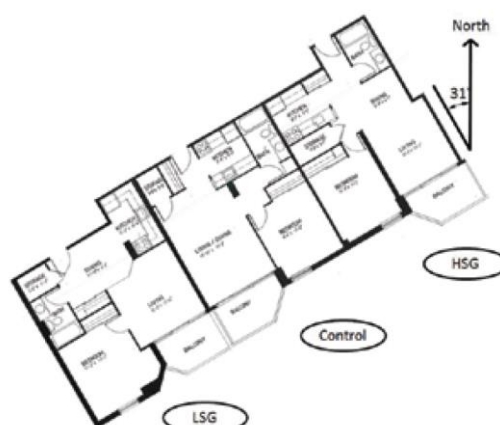
Figure 36. Test apartments facing east of south by 31 deg. Source: CMHC
