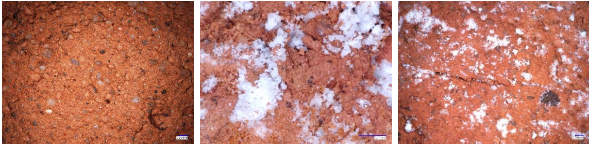
Fig. 5. The images of brick sample obtained from an optical microscope at the magnification of 50x, 150x and 500x. The images taken after 0, 15 and 20 cycles of exposure; larger cracks and salt crystals are visible.
