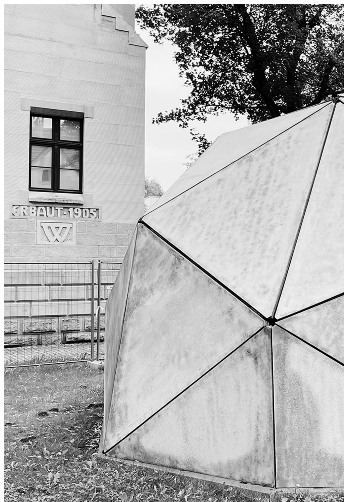
Ill. 3. Part of the ReSa project research model: panel coating based on a regular dodecahedron, author: Jakub Onyszkiewicz
