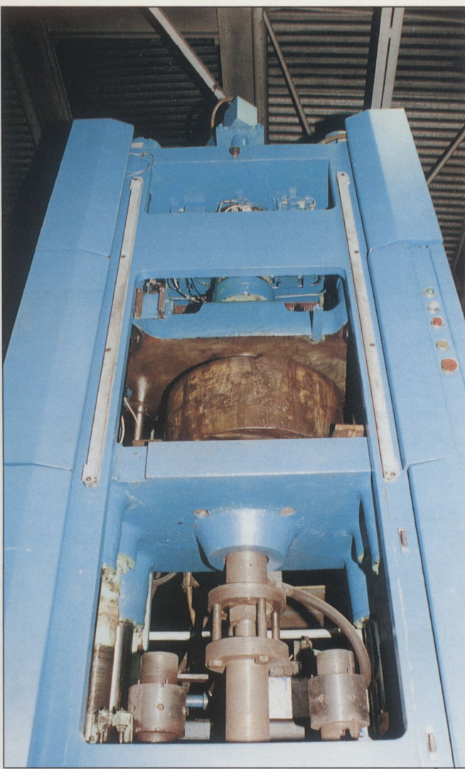
Pulsatory press PXP-100 type for powder products
