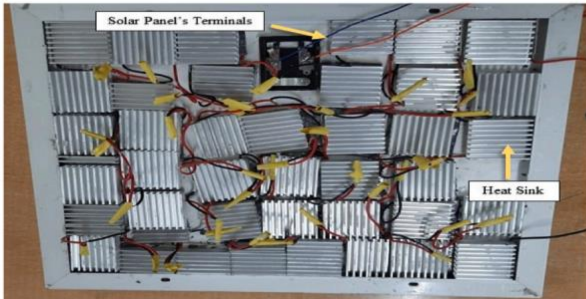
Figure 3-6. TEG combined PV/T system [42]
