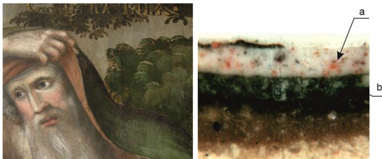
Fig. 3. A fragment of the wall painting of the southern wall with the use of verdigris pigment (a – lead bleach, ocher, b – lead bleach, green copper pigment verdigris)
