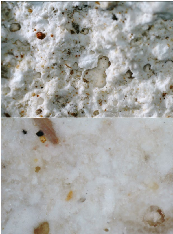
Fig. 10. Top: fragment of plaster from the eastern wall of the stairwell in H1 house, image at X20 magnification; bottom: fragment of the mortar pointing the ashlars from the western wall of the stairwell, house H1, X200 magnification; photo by P. Zambrzycki.
