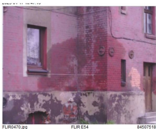
III. 16. Thermal imaging tests of façades of familok buildings in Bytom Bobrek – visible double temperature effect – severe dampness and the corner effect, unheated staircase. Photo by M. Krause-Świerczyńska, 01.2023
