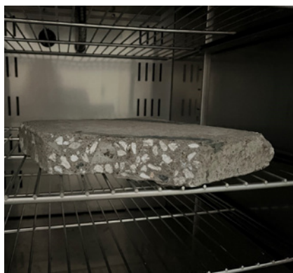
Photo 4. Cross-section of a sample of lightweight concrete with the addition of PCM, seasoned in a climatic chamber
