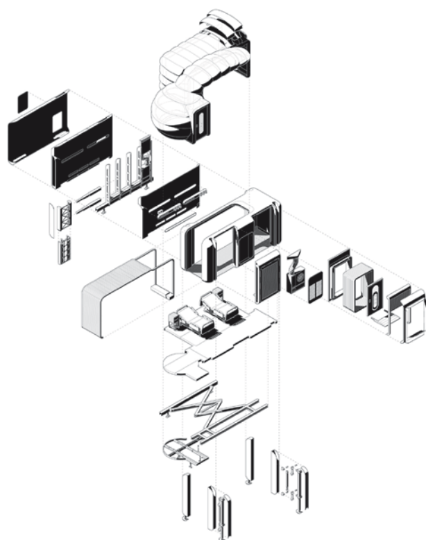
III. 6. An exploded axonometric diagram of one of the modules showing the components of the unit. Author: Przemysław Kielb
