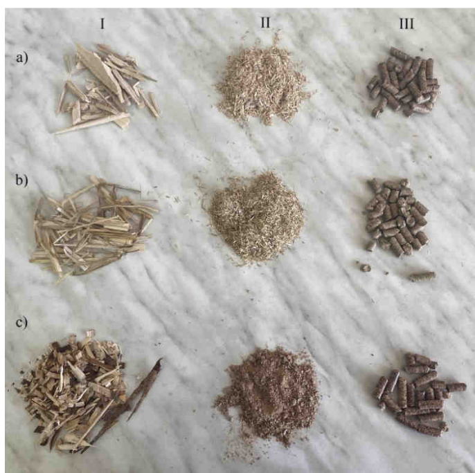
Fig. 1. Biomass selected for combustion tests in the binary fluidised bed: I) raw, II) crushed, III) pellet; a) sawmill, b) straw, c) willow
