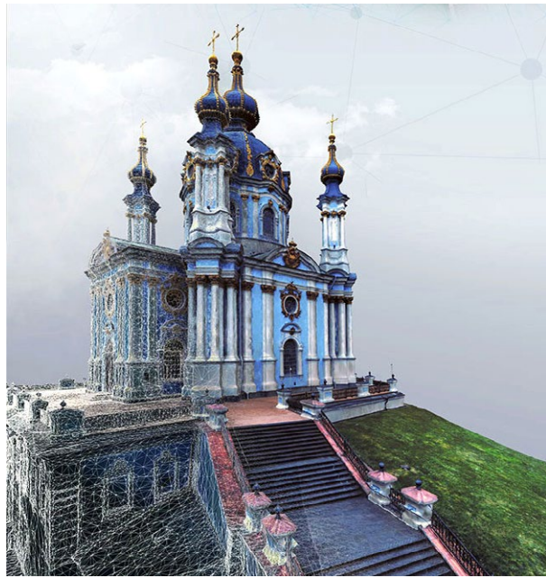
Fig. 6. The graphic model created using 3D scanning; figure by G. Kyselova
