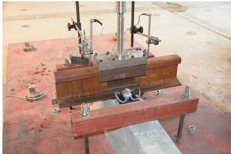
Fig. 5. Clamping force testing setup.
