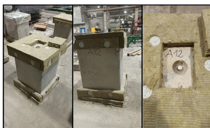
Figure 1. Column specimen with insulation covers
