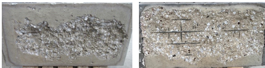
Figure 1: example of spalling comparison after ISO 834-1 fire: reference cement concrete (left) vs. low-carbon cement-based concrete (right)
