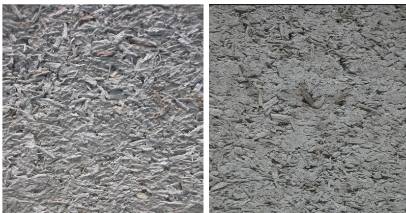
Figure 1. Surface of F800 and F1000 wood-chip based concretes
