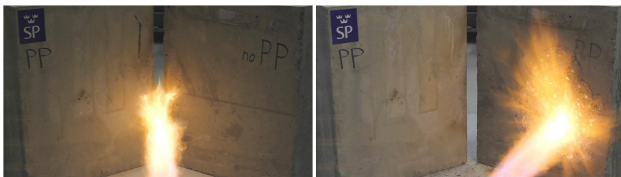
Figure 1. left: First heating of the corners of the specimens, no spalling recorded, right: Second heating of the centre of the specimen without a PP fiber addition, violent spalling occurred [1]
