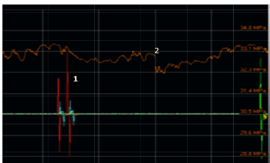
Fig. 4. Current characteristics of the injector coils (1) and the pressure in the "fuel rail" (2). Source: Own study
