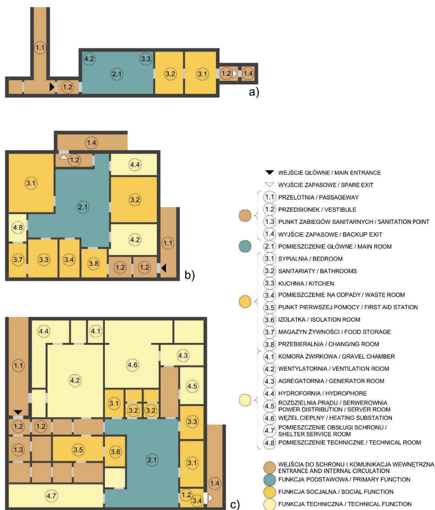
III. 2. Functional layouts of exemplary shelters, elaborated by A. Jörgen: a) shelter for 4-6 persons, b) shelter for 25 persons. c) training shelter at WAT
