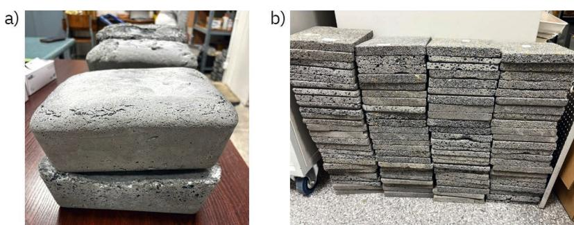
**Fig. 1.** Foamed geopolymers after demoulding (a) and slabs cut to size for testing insulation properties (b) (photo by Michał Łach)
