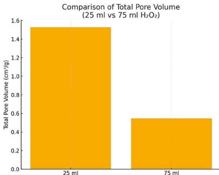
**Fig. 3.** Comparison of the total pore volume in materials produced with varying amounts of pore-forming agents
