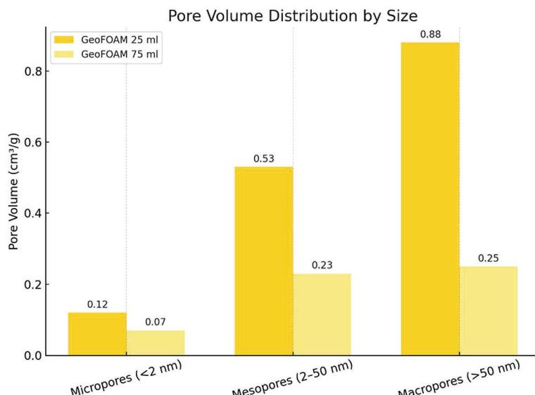
**Fig. 4.** Comparison of histograms showing pore volumes divided into micro-, meso-, and macropores for both series of foamed geopolymers (GeoFOAM 25 ml vs GeoFOAM 75 ml)
