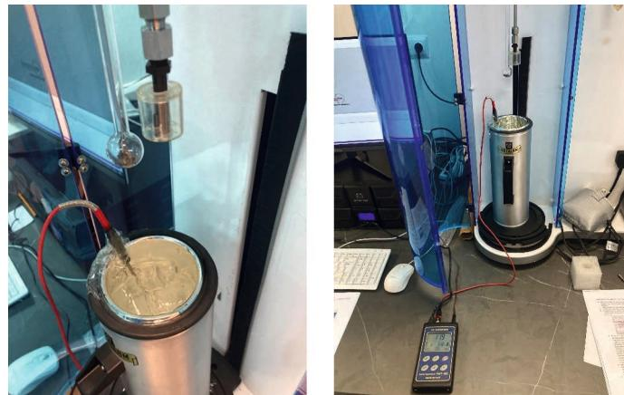
The pore size distribution, total pore volume, and specific surface area were determined using mercury porosimetry with a PoreMaster 33 device (Anton Paar GmbH, Graz, Austria). To cover the full range of pore sizes, the tests were conducted in two pressure ranges – low and high – using separate measuring chambers.
