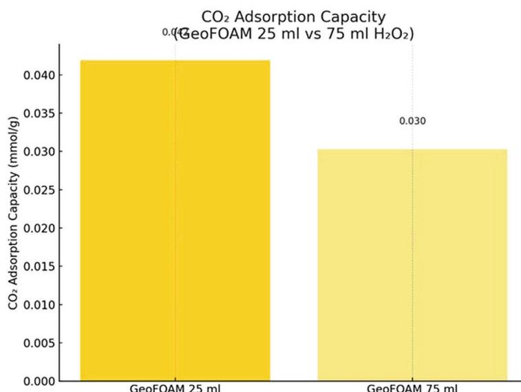
**Fig. 5.** Comparison of sorption capacities for foamed geopolymers, for variants with the addition of 25 ml H<sub>2</sub>O<sub>2</sub> and 75 ml H<sub>2</sub>O<sub>2</sub>
