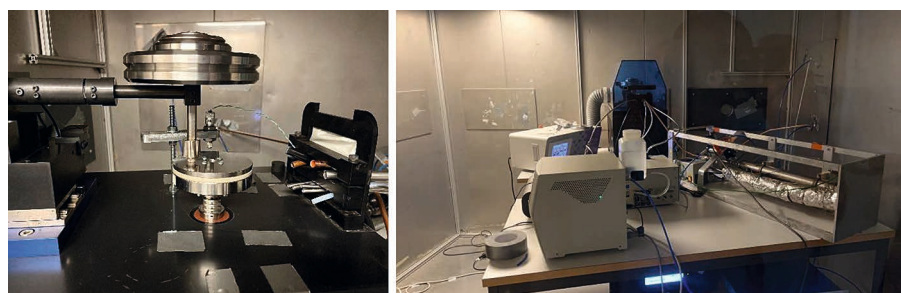
Fig. 12. Left: the pin in contact with the disc (where the contact force is applied by the dead weight at the top); right: blue polycarbonate enclosure on top of the pin-on-disc tribometer (source: D5.3)
