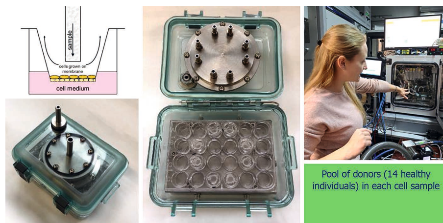
Fig. 16. Cell incubator for cell exposition during the tests (Cervena et al., 2025)
