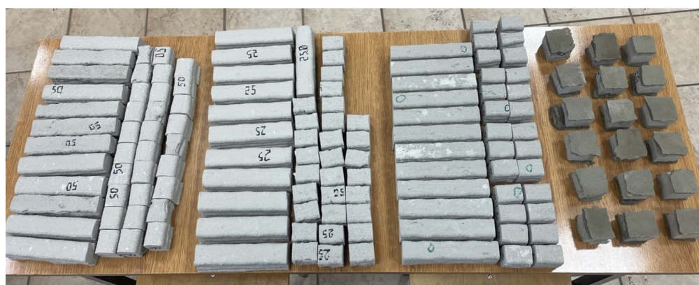
Figure 11. Printed specimens prepared for testing.
