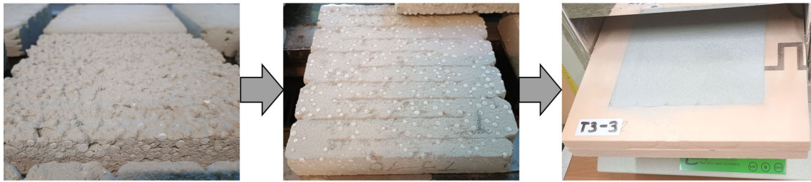
Figure 5. Schematic of specimen preparation for thermal conductivity testing of the 3D-printed material.
