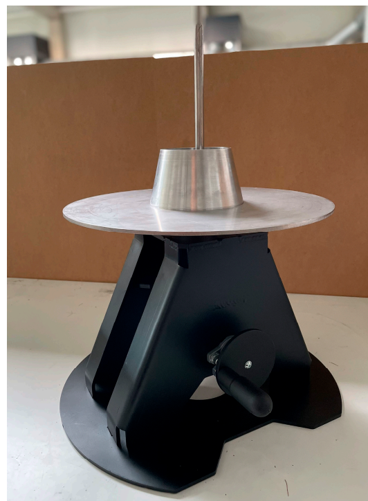
Figure 2. View of the flow table test device according to the PN EN 1015-3 standard.
