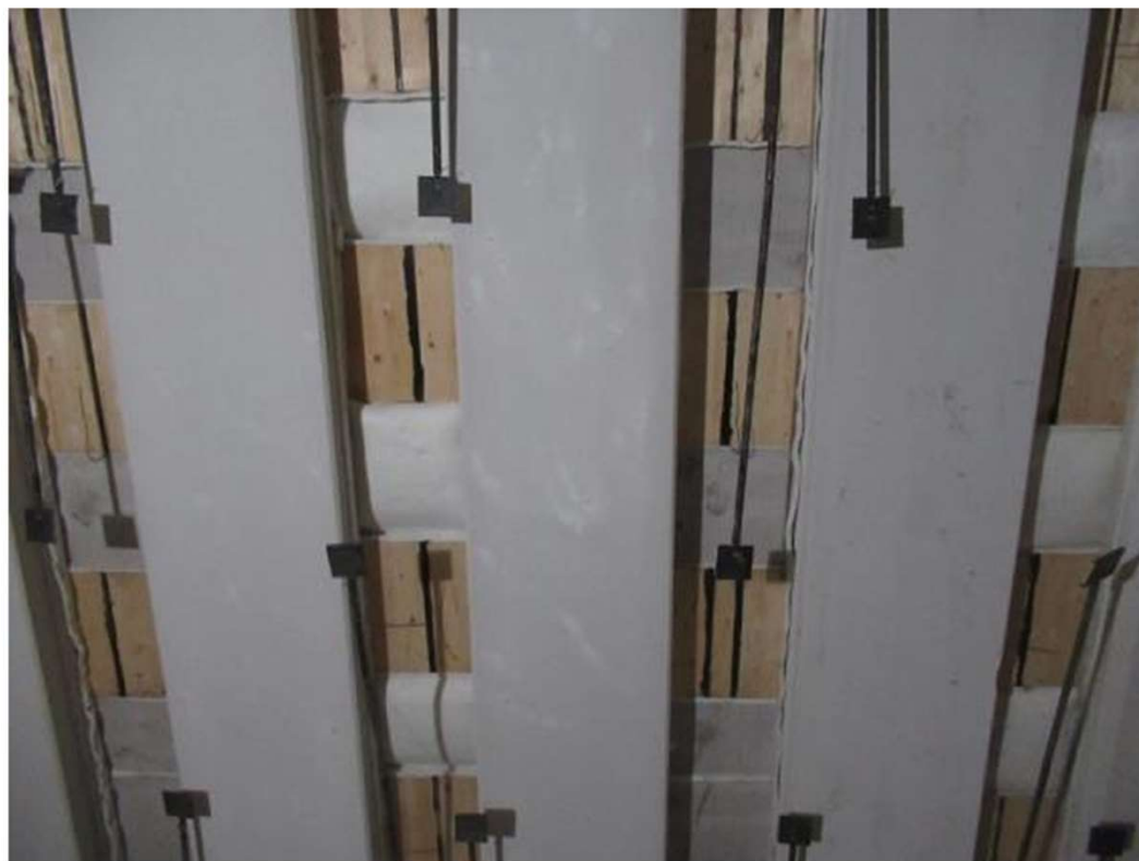
Photo A6.46: Positioning of plate thermocouples within the furnace below the specimens ( photo archive 049506d-234 )
