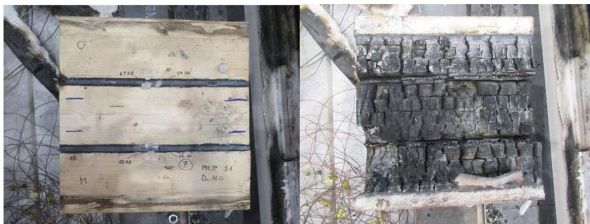
Photo A6.55: Specimen 7 after the fire resistance test – unexposed side (left) and exposed side (right) (photo archive left: 049506d-501 and right:049506d-502)
