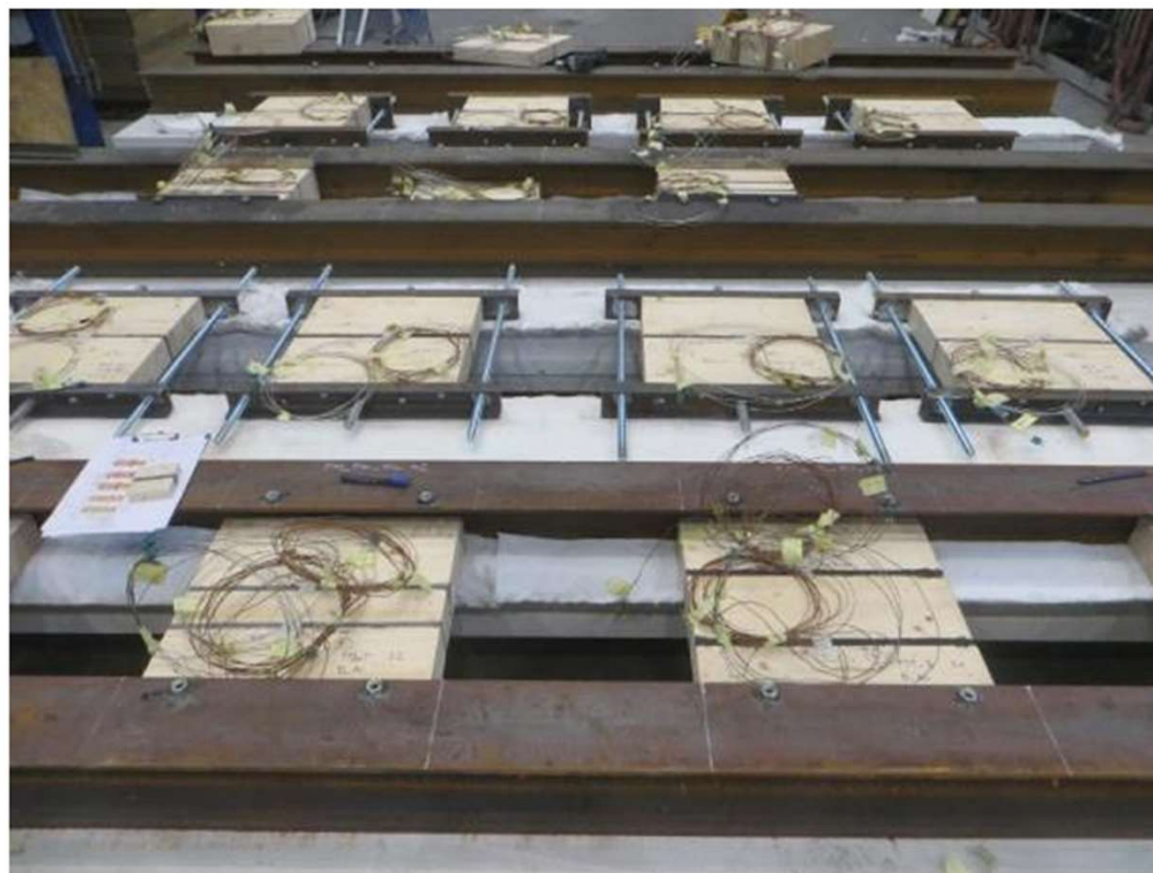
Photo A6.42: Positioning specimens on the supporting structure on the furnace frame ( photo archive 049506d-156 )
