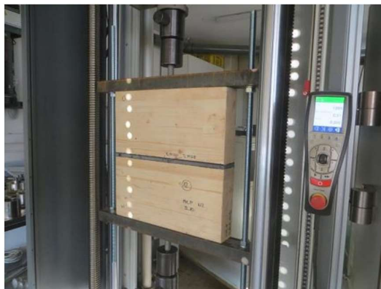
Photo A6.22: Mechanical loading of specimen no. 12 in tension (photo archive 049506d-069)
