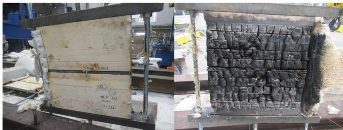
Photo A6.60: Specimen 12 after the fire resistance test – unexposed side (left) and exposed side (right) (photo archive left: 049506d-447 and right:049506d-448)
