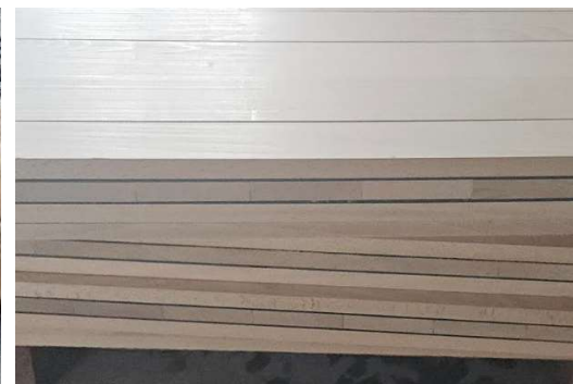
Figure 4: Hardwood-Based Composites with flexible polyurethane adhesive joints
