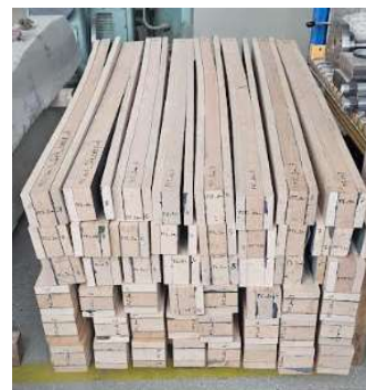
Figure 4: Hardwood-Based Composites with flexible polyurethane adhesive joints
