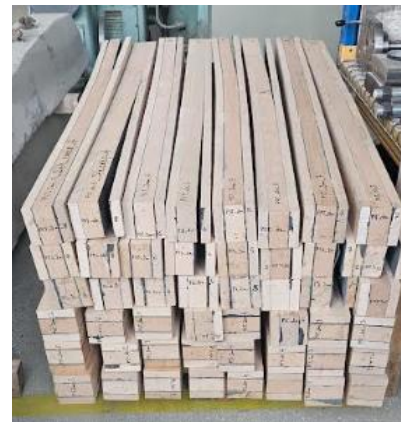
Figure 4: Hardwood-Based Composites with flexible polyurethane adhesive joints
