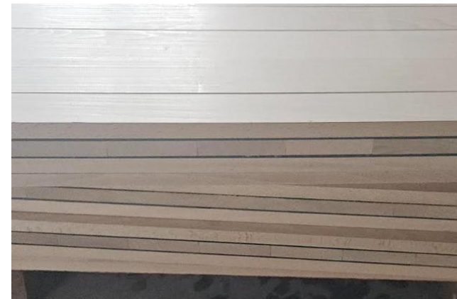
Figure 4: Hardwood-Based Composites with flexible polyurethane adhesive joints
