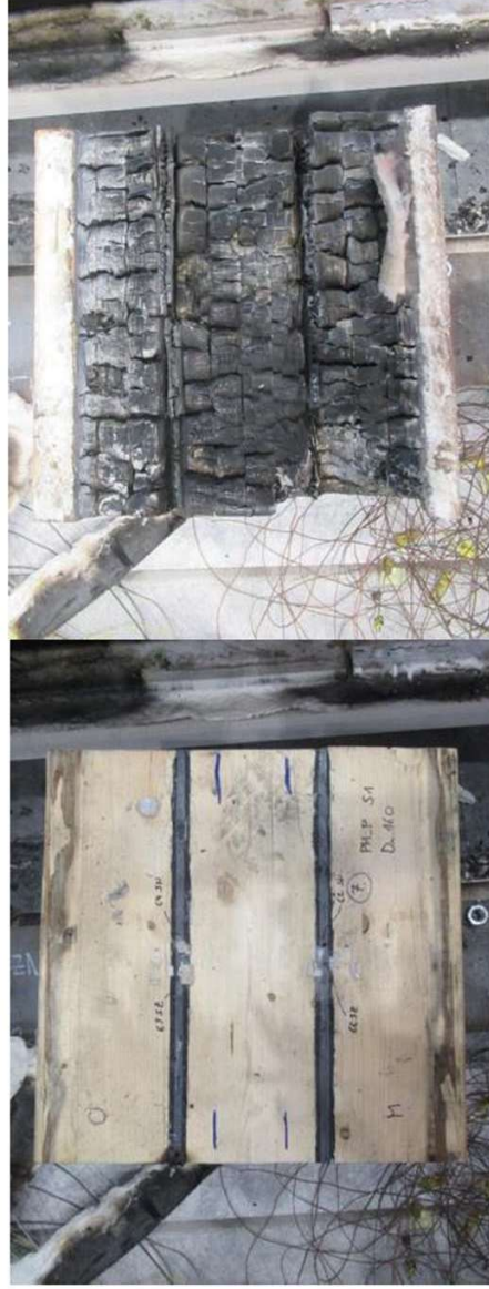
Photo A6.55: Specimen 7 after the fire resistance test – unexposed side (left) and exposed side (right) (photo archive left: 049506d-501 and right:049506d-502)
