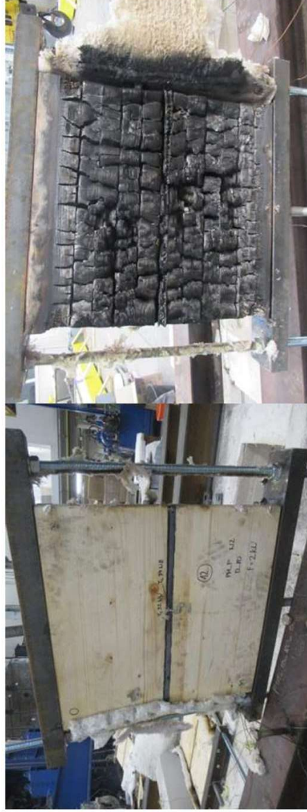
Photo A6.60: Specimen 12 after the fire resistance test – unexposed side (left) and exposed side (right) (photo archive left: 049506d-447 and right:049506d-448)
