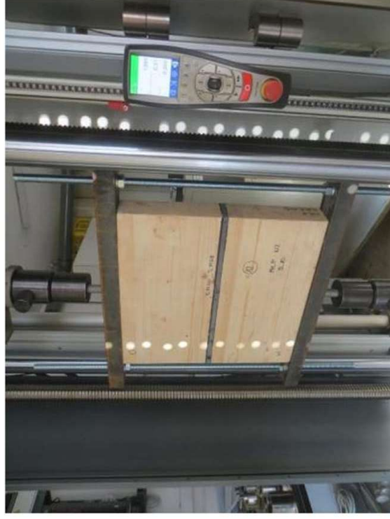
Photo A6.22: Mechanical loading of specimen no. 12 in tension (photo archive 049506d-069)
