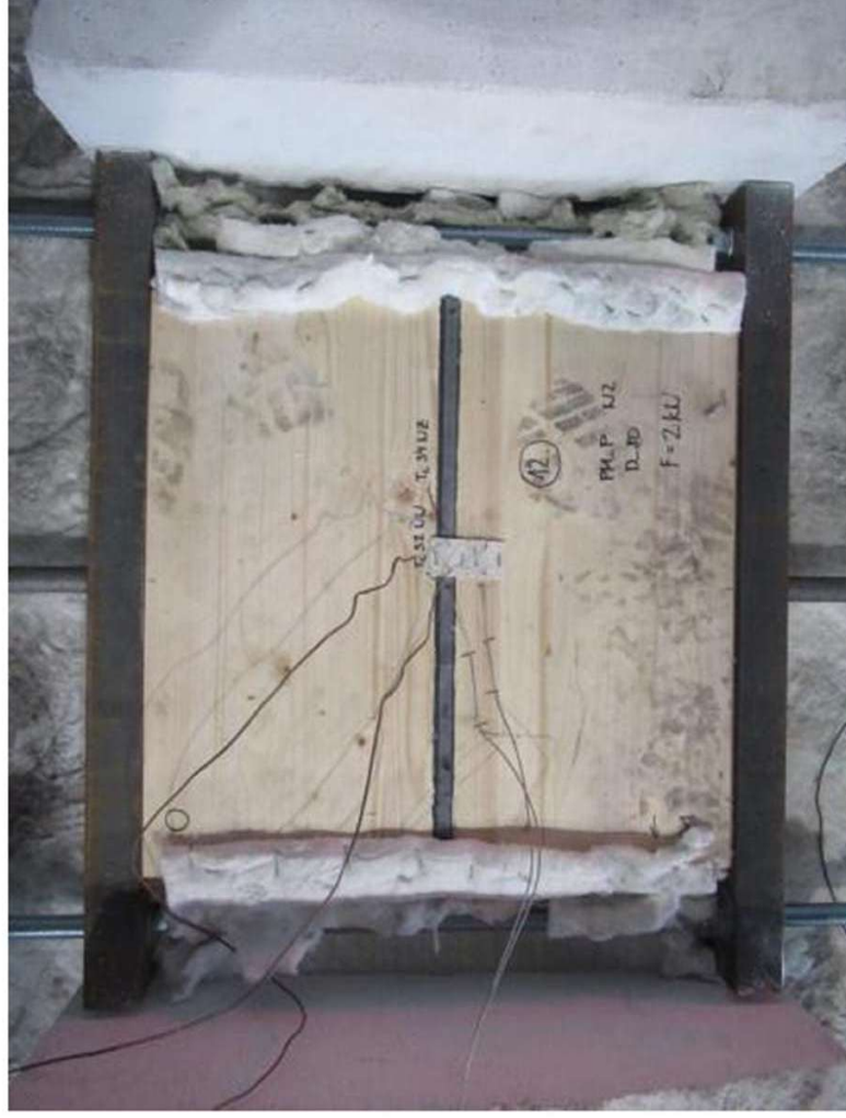
Photo A6.37: Thermocouple placement in specimen no. 12 (photo archive 049506d-270)
