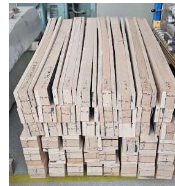
Figure 4: Hardwood-Based Composites with flexible polyurethane adhesive joints
