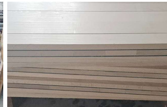
Figure 4: Hardwood-Based Composites with flexible polyurethane adhesive joints
