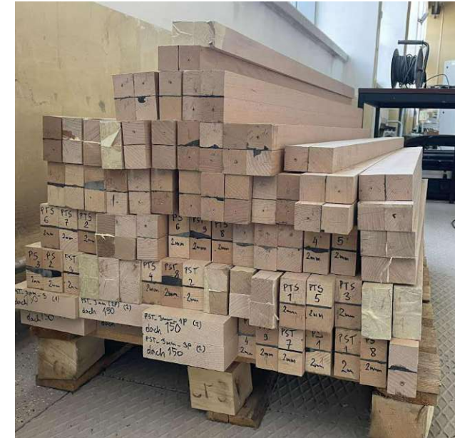
Figure 9. View of samples for four-point bending
