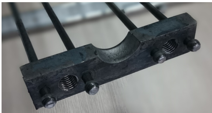
Fig. 2. Anchor block with prestressing rods with heads shaped using the BBRV method. Photo: authors' own elaboration
