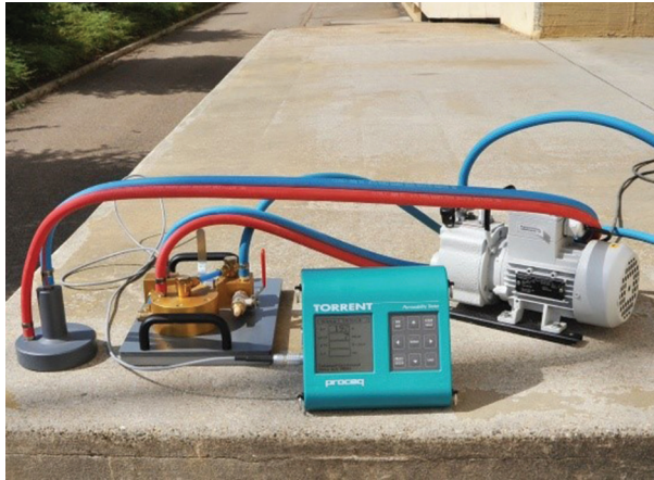
Fig. 8.5. Torrent air permeability test setup [15]
