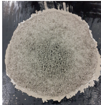
Fig. 3.2. Unstable concrete mix (i.e. severe segregation occurrence)
