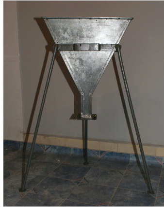
Fig. 3.3. V-funnel equipment according to EN 12350-9
