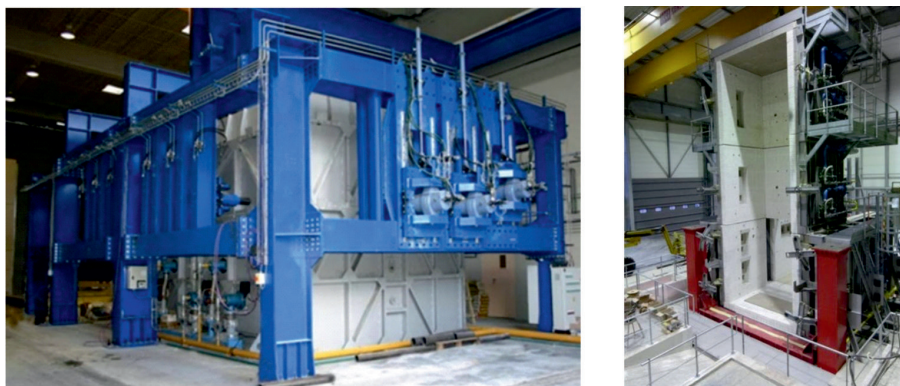
Fig. 6.6. Full-scale furnaces. Left: Promethee (CERIB, France); right: VULCAIN (CSTB, France)
