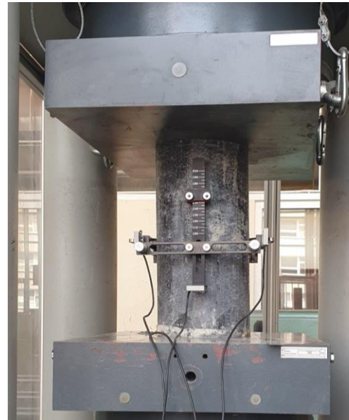
Figure 10. Testing the modulus of elasticity of samples.
