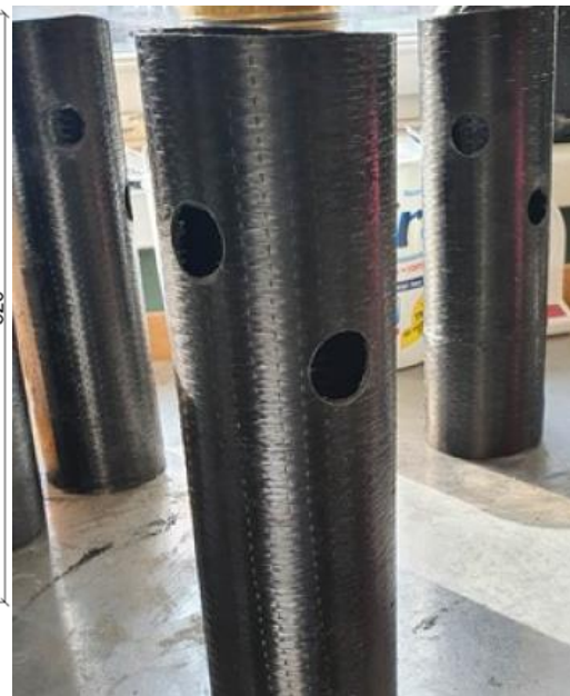
Figure 7. Example of perforation inner CFRP tube.
