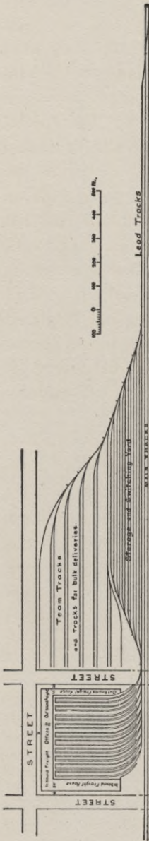
Fig. 142. Local Freight Yard.
